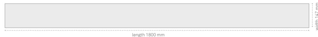
**öko skin flex:** In addition to the standard size of 1800 x 147 mm other formats within a width of 105 to 302 mm and within a length from 600 to 2400 mm are available on request.
